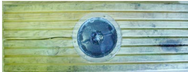
Figure 1 - Damage of SolarEye 80 product in decking following a compressive load of 600kN
