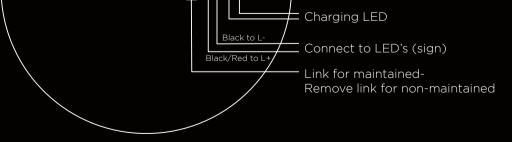
Charging LED - to be wired into LED Driver D+ & D-LED Wire - to be wired into the LED Driver L+ & L-Earth Wire - attach to the LED Driver fixing screw 240v supply to be wired to LED Driver L & N
