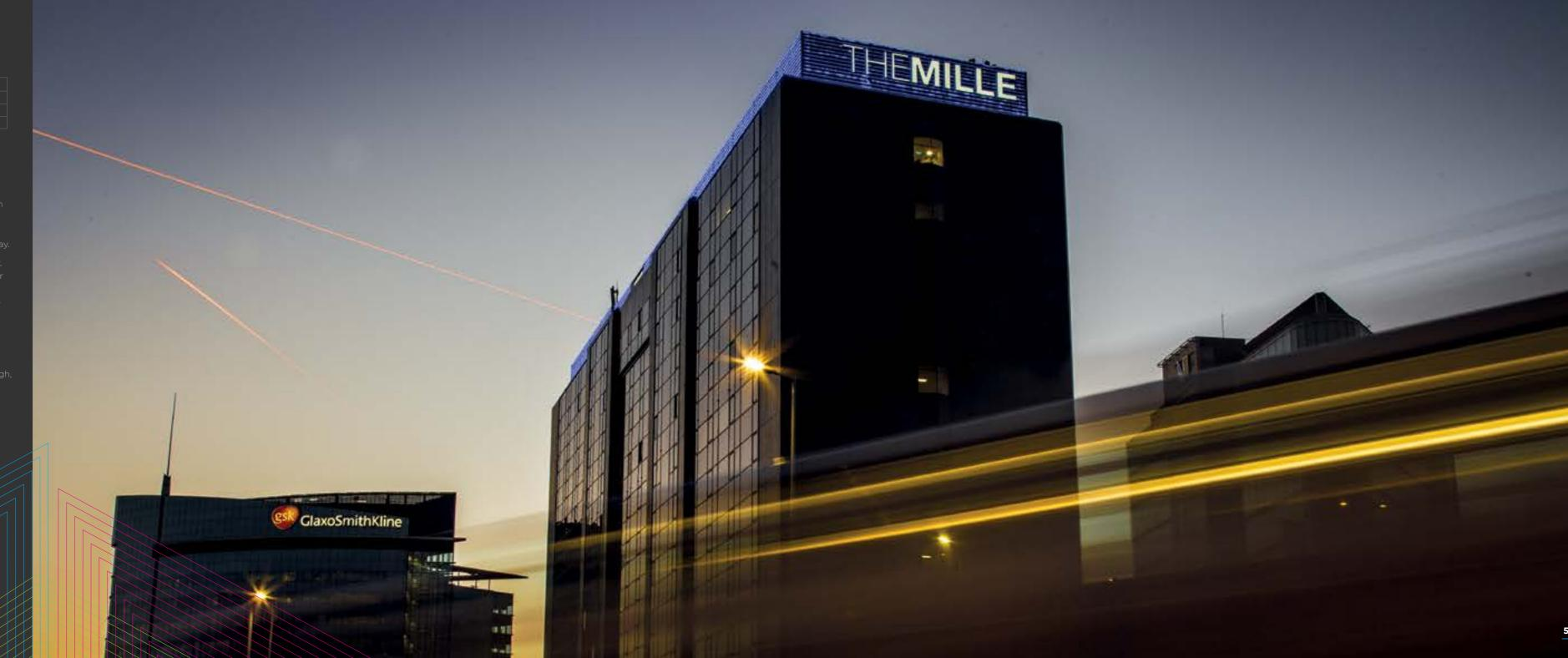
THE TECHNICAL DETAIL: For the challenging exterior signage, we created built-up, back-to-back letters with bonded-in polycarbonate faces that would withstand the high wind loads they'd face and created enclosures for remote switchgear to enable easy access for maintenance.
