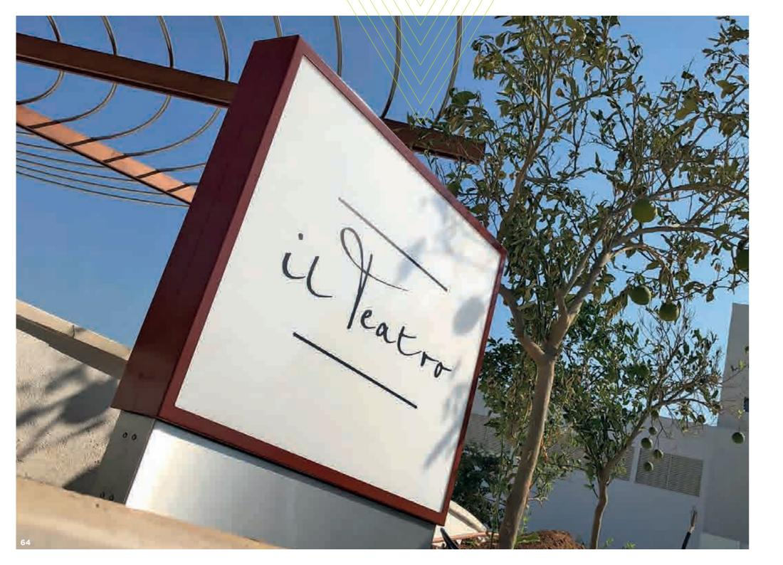
THE TECHNICAL DETAIL: The resort's external signage elements comprise branded entrance, directional and wayfinding signage and safety notices. Materials for the illuminated totem sign scheme include stainless steel subframes, stencil-cut aluminium trays that featured a specialist paint finish, push-through acrylic lettering and SloanLED illumination to set the scene for an unparalleled guest experience.
